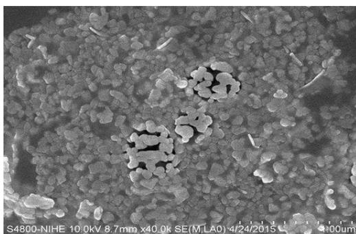
Figure 4. SEM pic of BiFeO<sub>3</sub> synthesized under optimal conditions.
