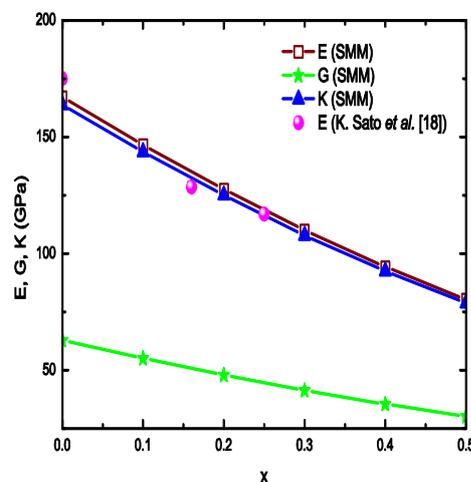
**Figure 4.** The dopant concentration dependence of Young's, bulk, shear moduli at the room temperature. The experimental results [18] are presented for comparison.
