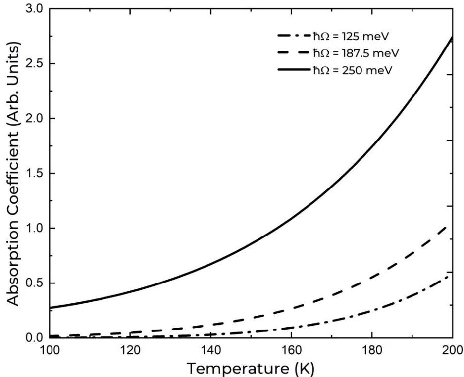
**Fig. 1.** The dependence of  $\alpha$  on  $T$  at 3 different values of photon energy  $\hbar\Omega$
