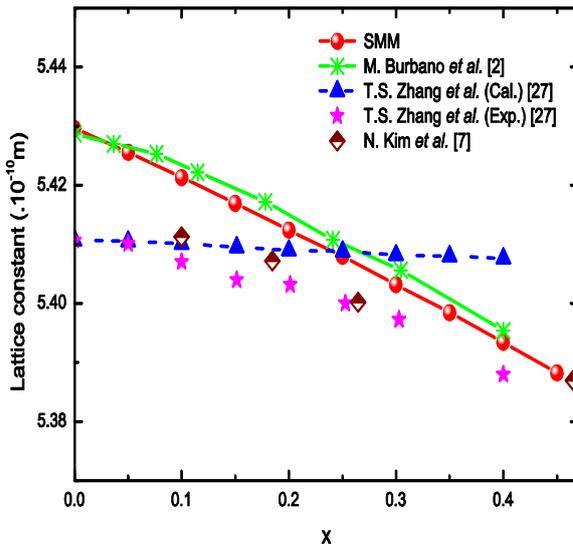
**Figure 1.** The dopant concentration dependence of lattice constant at  $T = 300\text{K}$ . The other theoretical [2, 27] and experimental [7, 27] results are presented for comparison.
