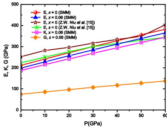
**Figure 6.** The pressure dependence of Young's, bulk, shear moduli at various dopant concentrations,  $x = 0$ ,  $x = 0.06$ . The results using LDA and LDA+U methods [15] are presented for comparison.
