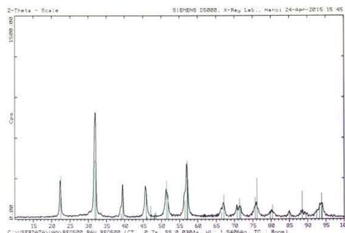
Figure 5. X-ray diffraction pattern of BiFeO<sub>3</sub> samples synthesized at optimal conditions
