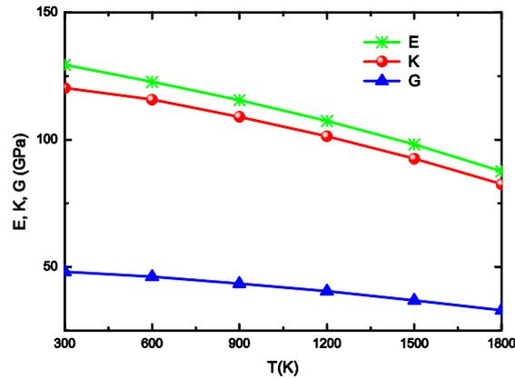
**Figure 5.** The temperature dependence of Young's, bulk, shear moduli of YDC crystal.
