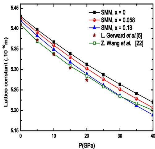
**Figure 3.** The pressure dependence of lattice constant at various dopant concentrations,  $x = 0$ ,  $x = 0.06$ ,  $x = 0.13$ . The experimental results [5, 22] are presented for comparison.
