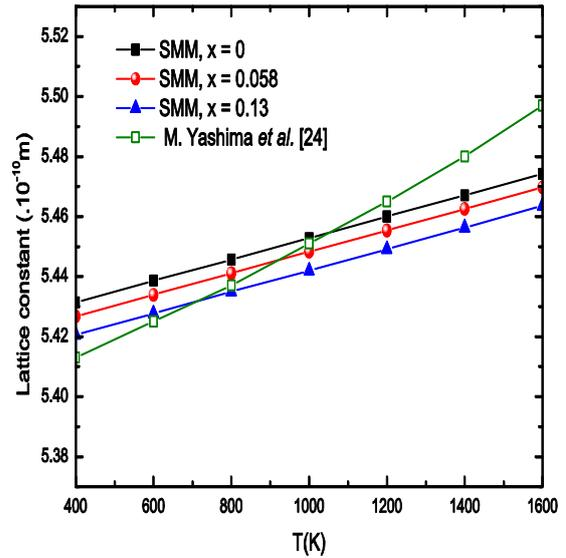
**Figure 2.** The temperature dependence of lattice constant at various dopant concentrations,  $x = 0$ ,  $x = 0.06$ ,  $x = 0.13$ . The experimental results [24] are presented for comparison
